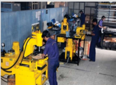
Hydraulic Bus bar Fabrication
